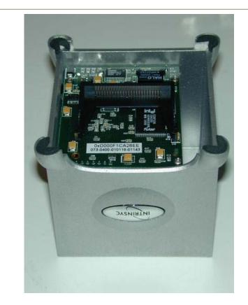
One good reason for leaving the CerfBoard exposed at the bottom of the cube is to allow access to its CompactFlash slot, which can be outfitted with a variety of expansion functions. Because of the exposure of its internal electronics, the CerfCube comes with an antistatic bag and a wrist strap for handling.
